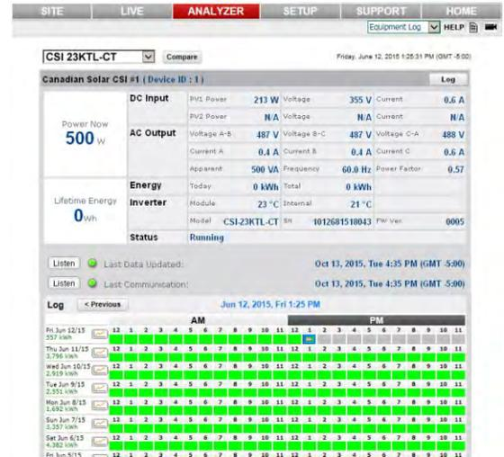
Fig 14 Detect intermittent internet connection from weak cellular or down land lines with the 30 day Communication
